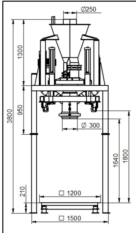
Weigh N Pack's Jumbo bag filling system is designed for filling of powder, granules, and other similar products which has good flowability character. As during filling operation material will not get any mechanical movement in case of filling of material with poor flowability (material with sticky nature) there will be need of another filling technology.
